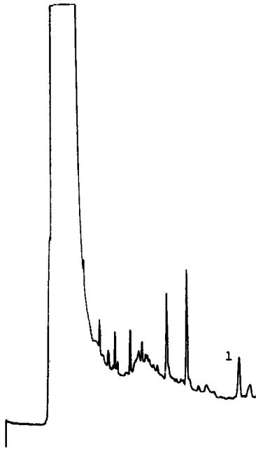
Figure 2: SFC chromatogram of a whole blood extract of a bone marrow transplant patient with about 228 \mu\text{g/L} of CsA at 18.4 min. Pressure programming from 100 to 300 atmosphere at 10 atmos/min. Peak identification: 1, CsA.
