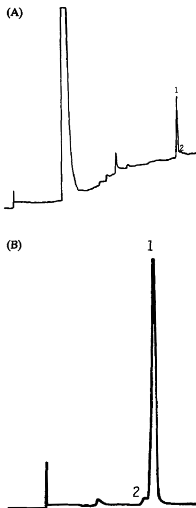
Figure 4: (A) SFC, and (B) HPLC chromatograms of FK 506. Peak identification: 1, FK 506; 2, FK 506 tautomer.
